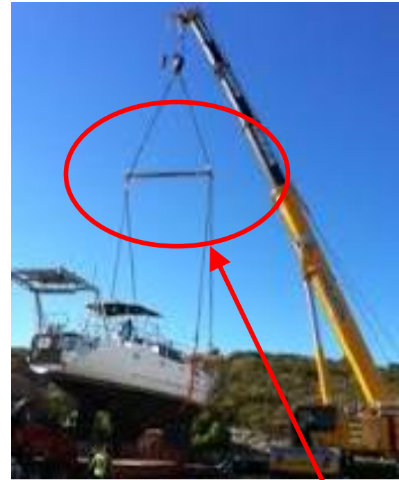
A spreader bar stops the load straps from pinching the hull
